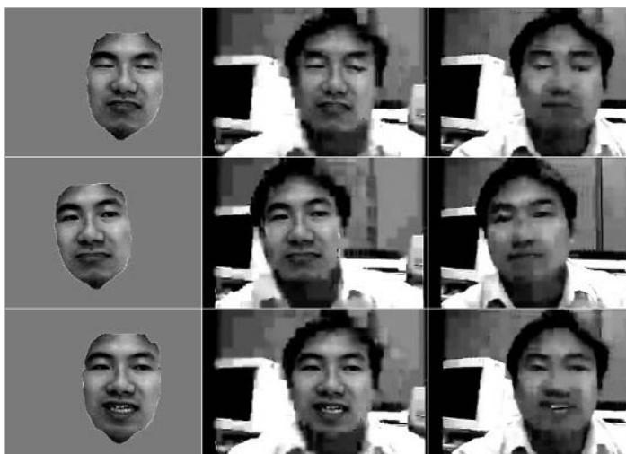
Figure 9. (a) The synthesized face motion; (b) The reconstructed video frame with synthesized face motion; (c) The reconstructed video frame using H.26L codec.
