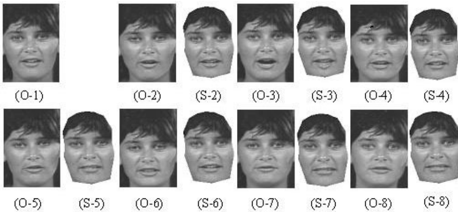
Figure 13. Facial animation using the face model of low complexity: (O- ) Original images; (S- ) Synthesized images.
