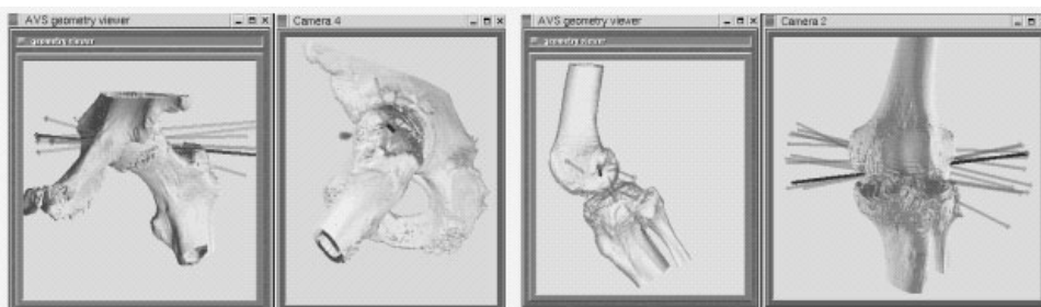
Figure 2. Joint kinematics. Left: Hip joint during a motion of flexion; Right: Knee joint flexion. Helical axes of motion are displayed, as well.
