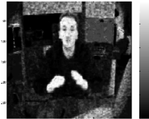
Figure 19. Moving hand segments after morphological reconstruction.
